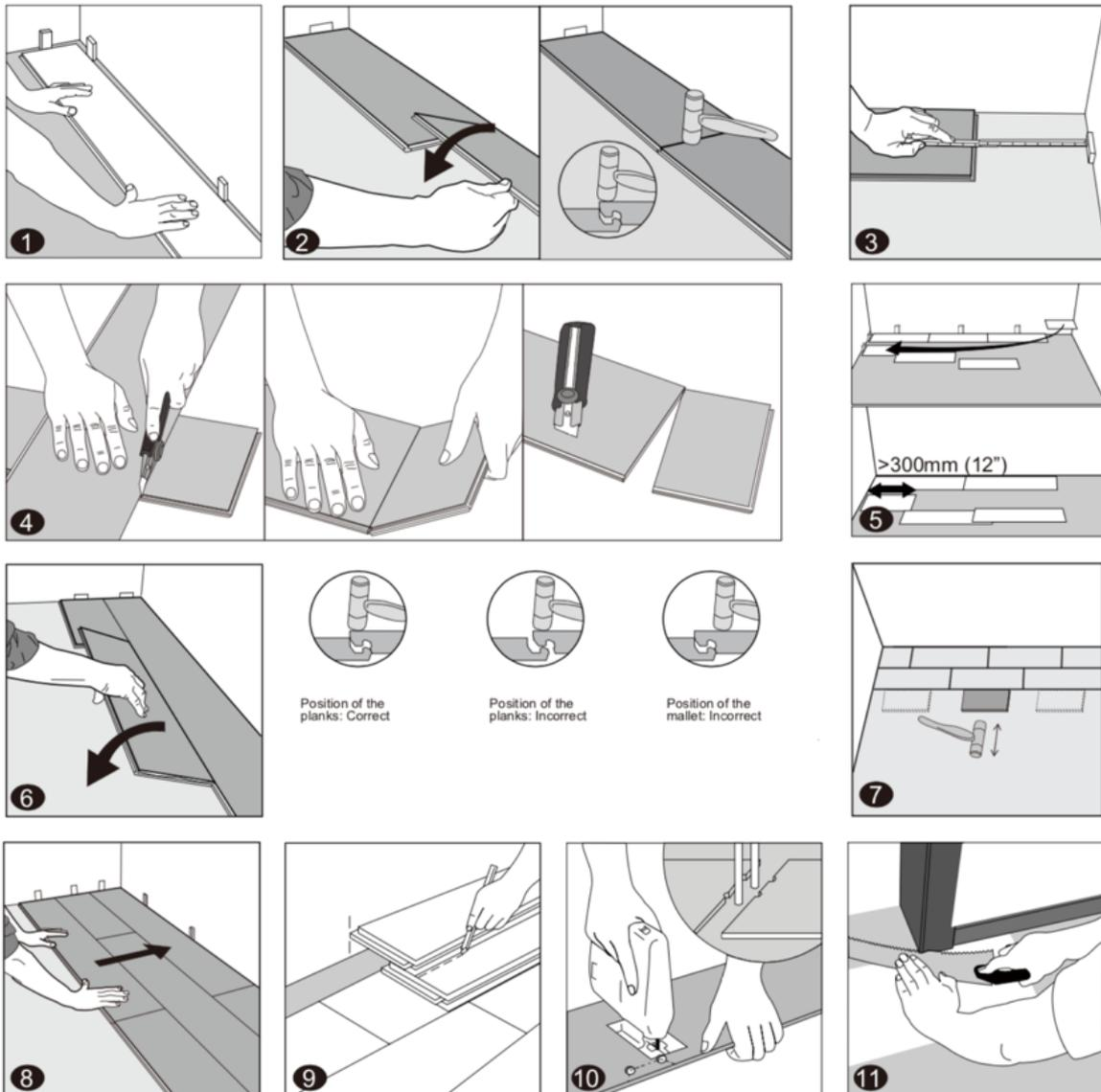
1. **First row, first plank:** After thoroughly cleaning the subfloor, you should begin laying from left to right. Position the first plank so that grooved edge is facing you. Place the floorboard 1/2" / 10 mm mm from the left wall. Use spacers between the wall and the floorboard.
