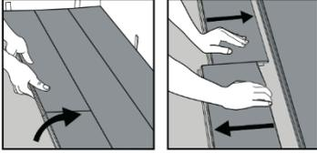
Separate the whole row by lifting it up delicately at an angle.
