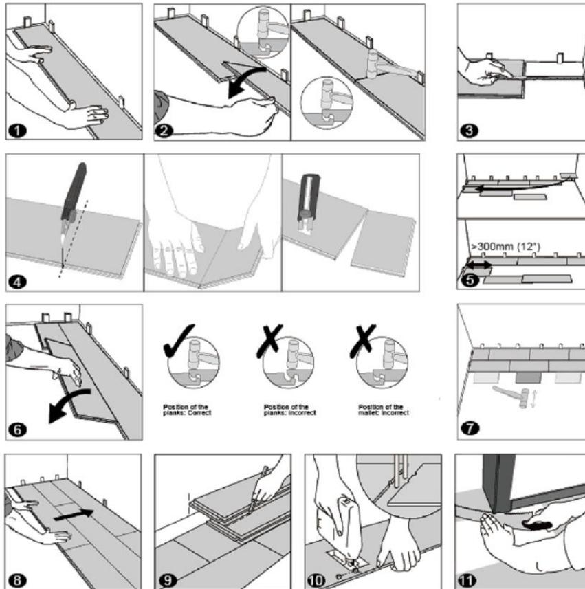
1. **First row, first plank:** After thoroughly cleaning the subfloor, you should begin laying from left to right. Position the first plank so that grooved edge is facing you. Place the floorboard 1/4" / 6 mm from the left wall. Use spacers between the wall and the floorboard.
